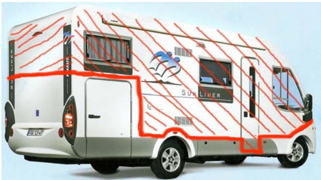
Figure 14: Investigated (insulated) indoor area of the motor home
